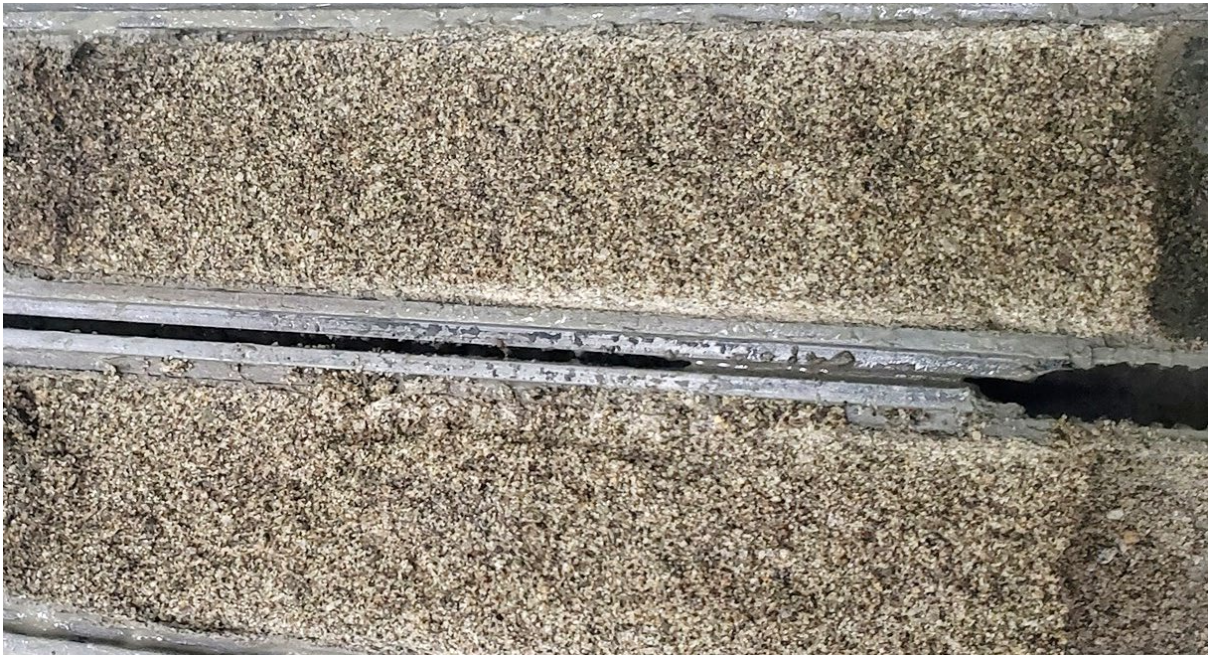
Plate 6 – ESU 4: Nonglacial Deposits Q pon | Very dense, fine SAND, trace silt | PG-2, S-9 @ 35 – 36½ feet.
