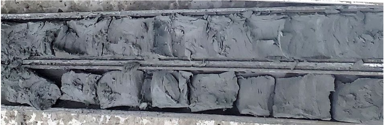
Plate 5 – ESU 3: Q ylc | Very stiff to hard, silty, lean CLAY to clay SILT | PG-2, S-6 @ 20 – 21½ feet.
