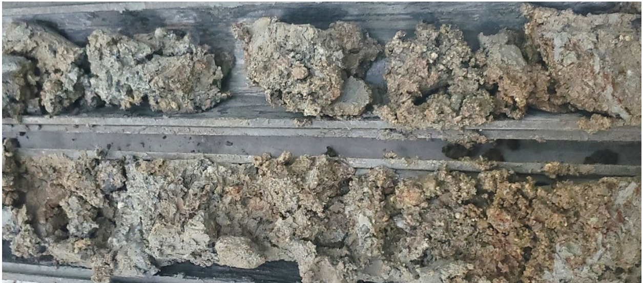
Plate 3 – ESU 1: Hf | Very loose to loose, silty sand | PG-2, S-2 @ 5 – 6½ feet.
